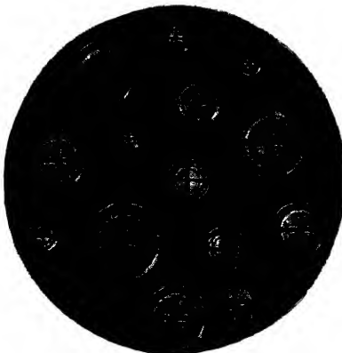
FIG. 161.—Spherulitic Crystals of the solid form of Cholesteryl Acetate, projected on the Screen in the Act of Growth (see p. 232) from the Doubly Refracting "Liquid Crystal" form
